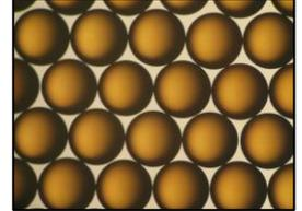
AMBERLITE HPR1300 H provides great mechanical strength and oxidative stability. It is ideally suited to the high flowrate demands of condensate polishing applications. The enhanced stability of this resin makes it suitable for the more challenging industrial applications or when more stringent water quality is required. In working and polishing mixed beds, it is a good choice when very low sodium leakage and conductivity is a chief concern.
