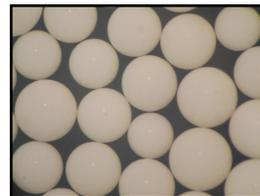
Weak base anion resins are well-suited for use with strong base anion resins to improve overall efficiency and throughput of a demineralization system. It effectively removes mineral acids and organics, reducing the ionic load on the strong base anion resin and also protecting it from organic fouling. The weak base anion resin increases a system's overall capacity to remove organics.
