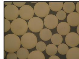
When AMBERLITE™ IRC83 H is operated in the Na-form, it will remove total hardness even in high salinity waters such as those in oilfield SAGD systems. When operated in the H-form, it will remove only the hardness associated with alkalinity—a weak acid cation resin operated in the H-form is well-suited for use with strong acid cation resins to improve overall efficiency and throughput of a demineralization system by reducing the hardness exposure on the strong acid cation resin.
