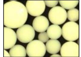
In industrial demineralization when operated in the OH-form, AMBERLITE SCAV3 Cl is ideally used as a polisher of remaining organics when placed after the anion vessel to meet the more stringent quality specifications for make-up water. Due to its strong base functionality, it will also have the ability to demineralize. When operated in the Cl-form, it can alternatively be used as a lead scavenger.
