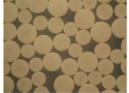
When operated in the H-form, it will remove only the hardness associated with alkalinity—a weak acid cation resin operated in the H-form is well-suited for use with strong acid cation resins to improve overall efficiency and throughput of a demineralization system by reducing the hardness exposure on the strong acid cation resin.
