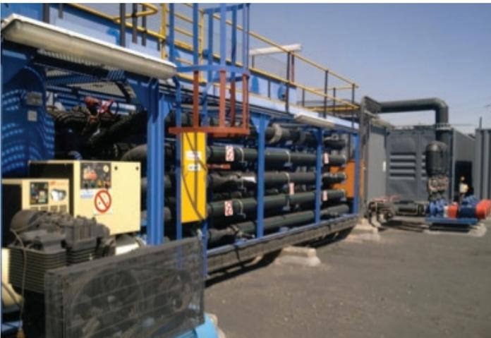
The mine stores high salinity and variable suspended solids (TDS 6000 mg/l, NTU 1-30) in an open pond on site. In order to remove suspended and dissolved materials from the wastewater, Dow partnered with a local OEM to rapidly deploy a modular containerized system. Dow UF and RO technology effectively helps to reject particles, colloids, suspended solids, oxidized Fe/Mn and microorganisms from the wastewater.
