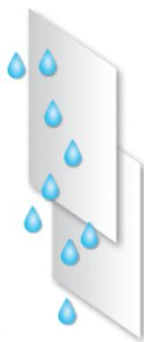
DuPont™ Tyvek® building wraps with proper overlap shed water away from the wall.
