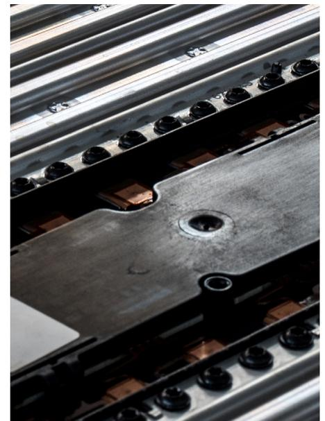
Due to temperature swings, the screws securing the coolant system to the battery pack made noticeable noise during expansion and contraction.
