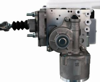
Electro-hydraulic braking (EHB) is a fast-growing technology that replaces older booster brake technology. The braking unit, as shown here, is controlled by electronic actuators that activate the brake hydraulics.
