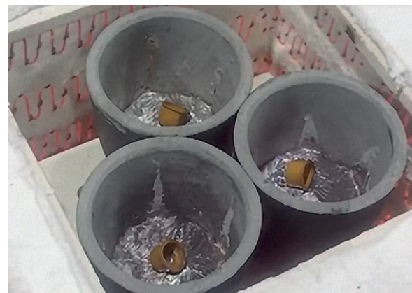
Figure 5: Vespel® Inserts Floating on the Surface of Melted Aluminum
