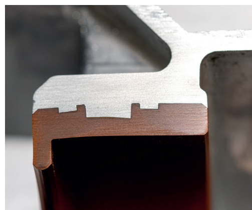
Figure 4: Cross section of bearing seat with Vespel® insert (© DuPont)
