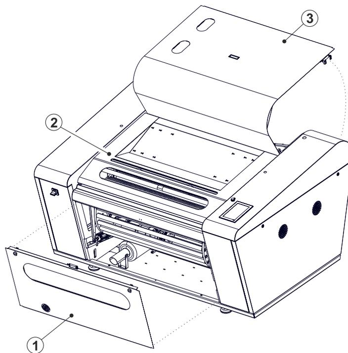
**i NOTE:** When the front cover, the top cover, or the rear door have been opened and closed, the processor will require that the error generated in the alarm menu is cleared and that the processor is initialized. This is to ensure that no plate is left inside the processor, and to re-establish safety circuits and correct processor conditions.
