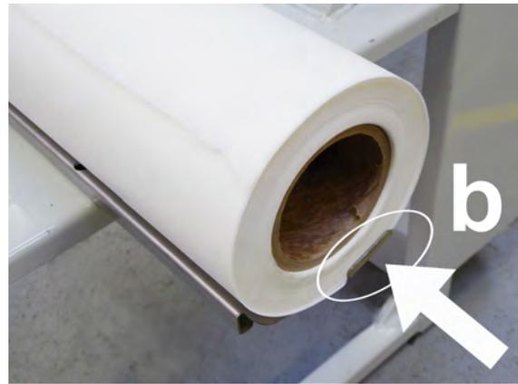
14. Remove any protection wrap from the new roll and check the material for any signs of damage.
