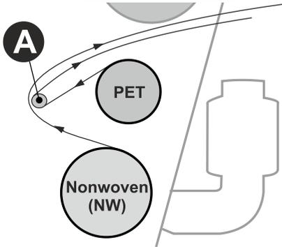
10. Straighten the nonwoven and PET into one layer and then make a triangular fold of the front edge and create a 'tip', still with the nonwoven and PET as one layer.
