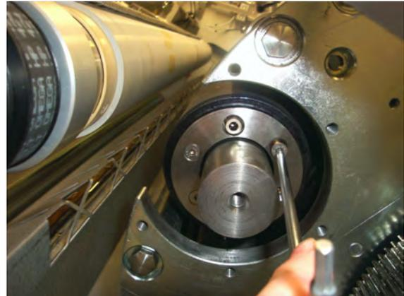
28. Mount the format cylinders support bracket. Use the allen key No 5.
