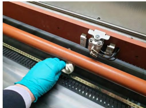
15. Once the visible section of rubber roller has been cleaned, replace the top cover in the down position.
