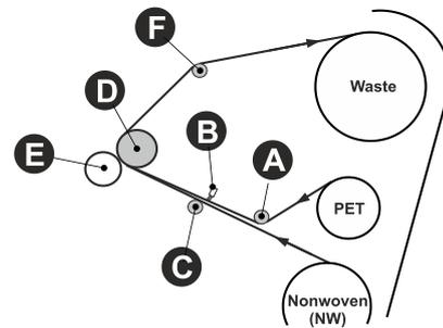
14. Lead the tip of the nonwoven/PET above the roller (F) and out, above the waste roller.
