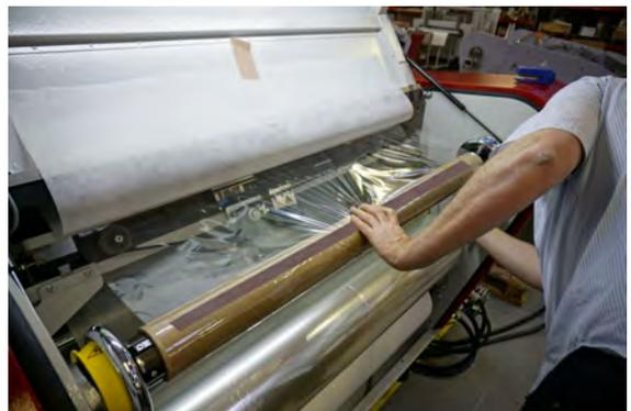
19. Mount another piece of double-side self-adhesive tape on top of the PET for mounting of the nonwoven.
