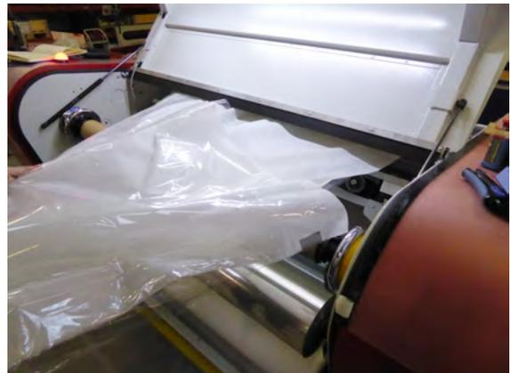
15. Cut off the ends of the nonwoven and PET and straighten the materials.
