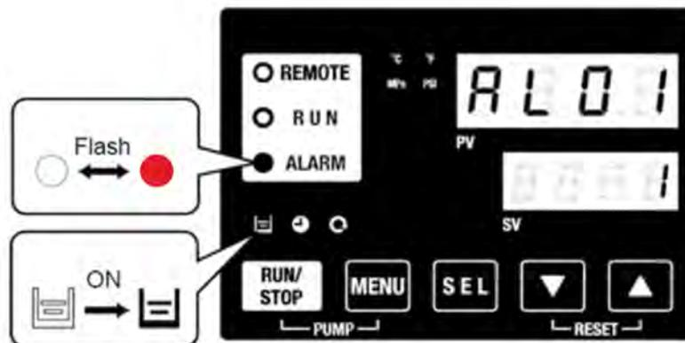
7. Reset the "AL01; Low tank level". Press the [RESET] key ([▼] and [▲] keys simultaneously) to stop the alarm buzzer.
