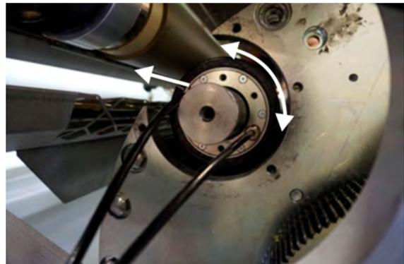
18. Keep pulling on the slip fit adapter along the format cylinder until it is fully removed.
