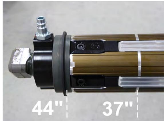
19. Mount the air shaft with the empty roll in the chuck bearings.
