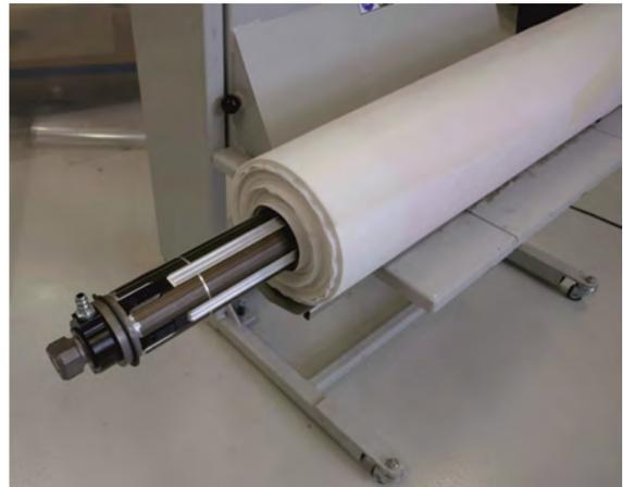
18. Position the roll according to the position marks for 44" or 37" roll as illustrated in the photo:
