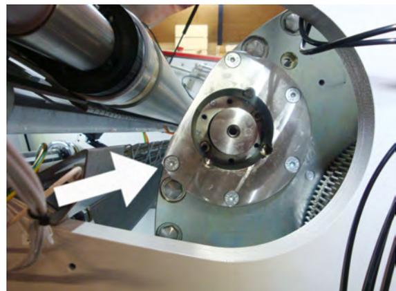
29. Mount the lift shaft delivered with the equipment and push the taper lock through the lift shaft and into the format cylinder until aligned with the front edge of the format cylinder's support bracket.
