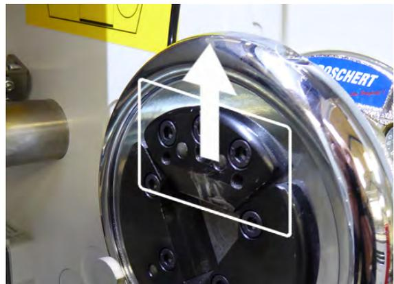
7. Unlock the chuck bearing in the left and right side of the roll by pressing the chuck bearing's top-edge outwards (away from the roll).
