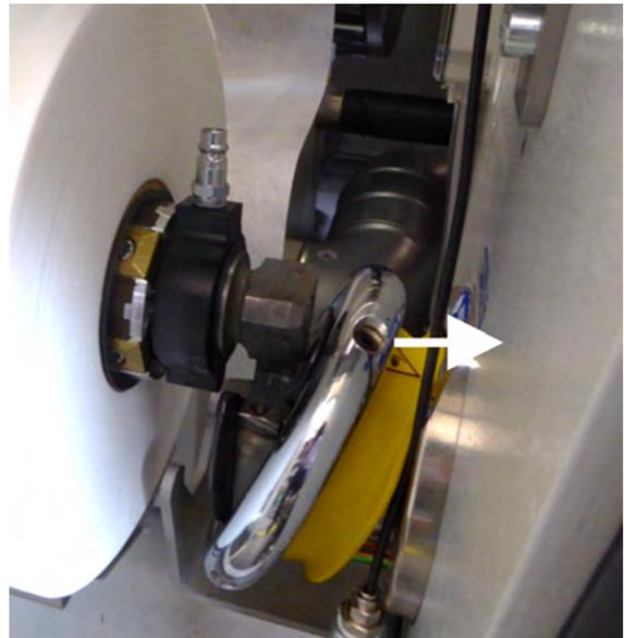
22. Ensure the air shaft's connection block is correctly positioned in the chuck bearing holder.
