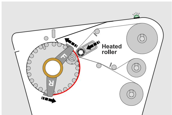
After each revolution, the heated roller retracts to avoid hitting the clamp arms.
