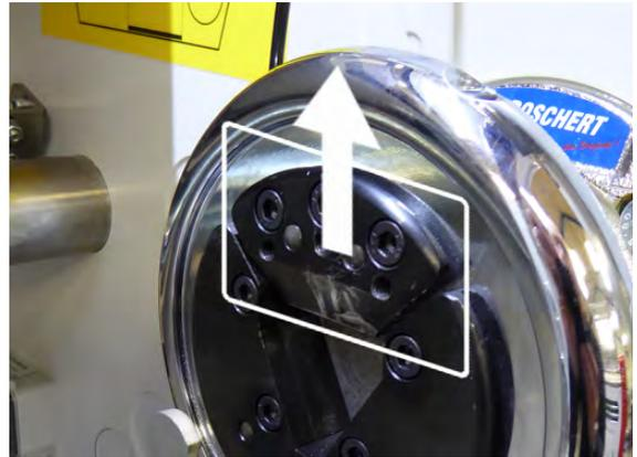
6. Unlock the chuck bearing in the left and right side of the roll by pressing the chuck bearing's top-edge outwards (away from the roll).
