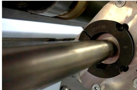
11. Dismount the format cylinders support bracket. Use the allen key No 5.
