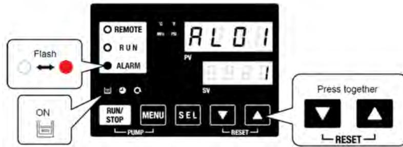
8. **To Stop:** Keep the [RUN/STOP] key pressed for approx. 2 seconds. The [RUN] lamp flashes (green) and continues the operation until the chiller is ready to stop. After approx. 15 seconds, the [RUN] lamp goes off and the chiller stops
