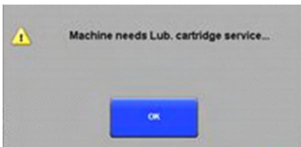
Each message is displayed in a separate pop up box (an example is shown above) and needs to be acknowledged separately. Any combination of all 3 messages can be displayed at one time (1, 2 or all 3). To acknowledge the reminders, select OK. When the service reminders are displayed please contact your local DuPont Service or local DuPont representative to organise a service visit immediately.
