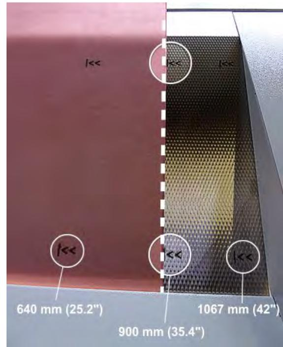
3. Gently push the plate into the entrance slot so that the front edge of the plate rests on the 2 front stops.
