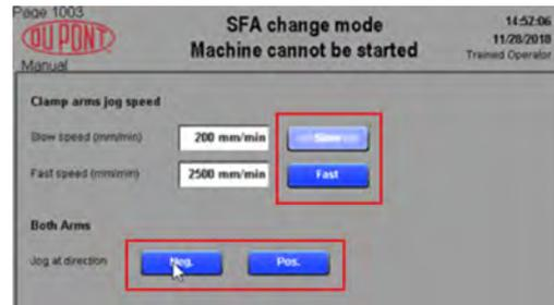
16. Use the Neg or Pos buttons with either the fast or slow button selected to rotate the rubber roller so that the next dirty section of the rubber roller is accessible.
