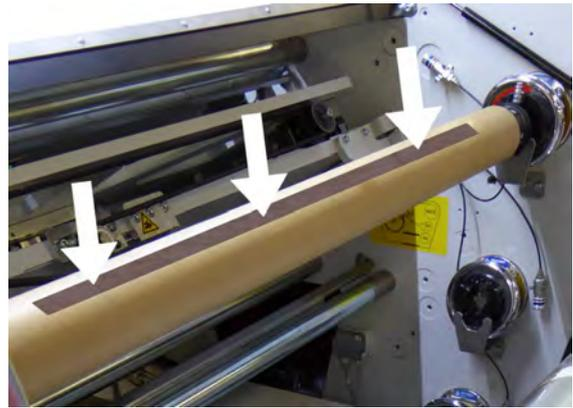
23. Loosen the PET from the top cover and mount it to the empty roll.
