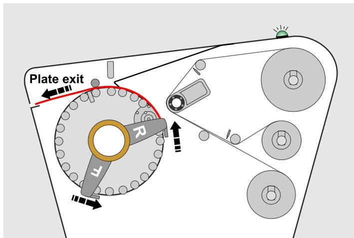
The plate will continue to exit the processor until the rear clamp arm stops in the eject position.
