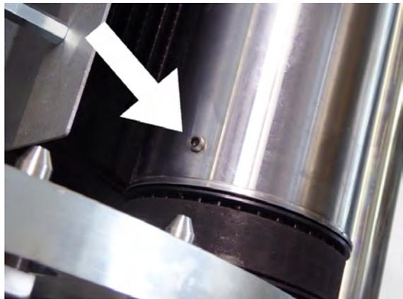
13. Mount the air hoses included with the tool kit in two fittings as shown.
