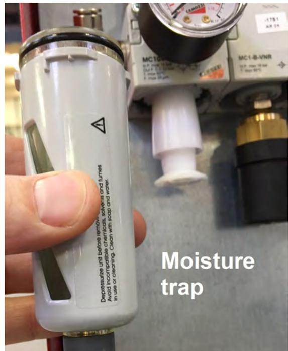
5. Unscrew the bottom part of the filter (see photo) and clean in water.
