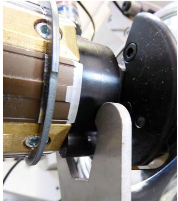
21. Lock the chuck bearings in left and right side by pressing the chuck bearings inwards (towards the roll).
