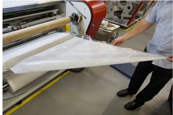
12. Lead the tip of the nonwoven/PET back inside the processor and underneath the anti-static brush (B) and above the roller (C).
