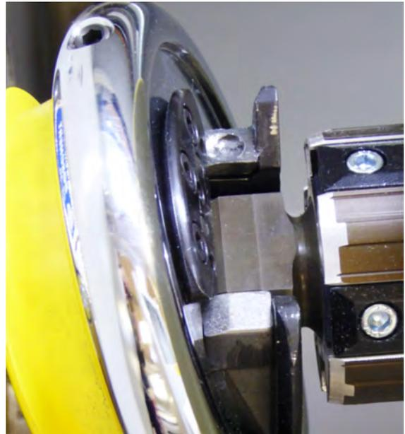
25. Lock the chuck bearings in left and right side by pressing the chuck bearings inwards (towards the roll).
