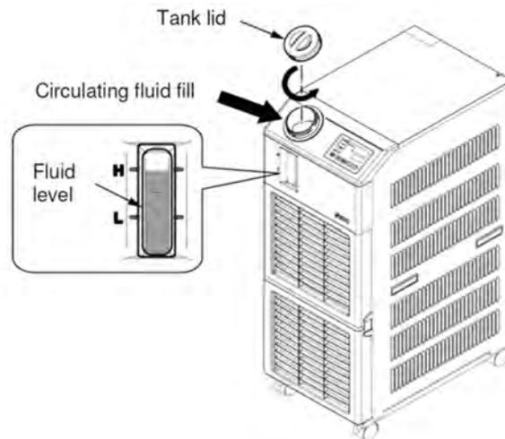
4. The chiller is to be filled with a mixture of clean water and anti-freeze. The specification for the anti-freeze is:
