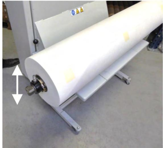
21. Push the lift table into the processor and position the air shaft directly above the chuck bearing.
