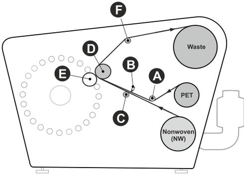
Correct threading of nonwoven, PET, and waste
