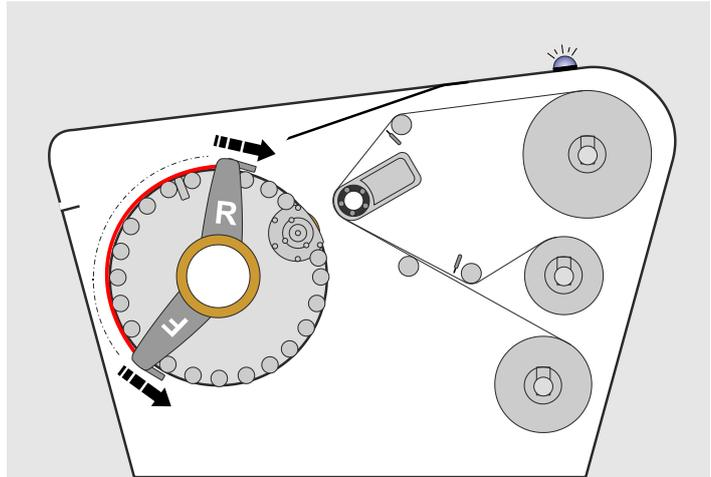
The front and rear clamp arms will now synchronize with each other and rotate the plate around the static drum. The stack light will flash green.
