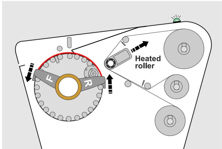
Once the full number of revolutions has been completed, the processor will automatically position the front clamp arm in the eject position.
