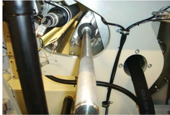
30. Align the 3 holes of the taper lock with the 3 holes in the cylinder support bracket.
