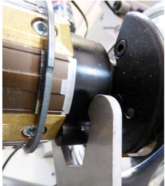
23. Slowly lower the lift table until the air shaft is resting in the chuck bearings.
