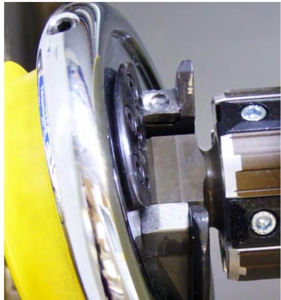
20. Ensure the air shaft's connection block is correctly positioned in the chuck bearing holder.
