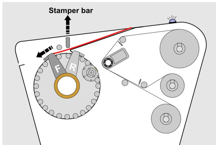
After about two seconds, the lay-down roller will drop onto the plate surface to keep tension on the plate as it is pulled around the static drum.
