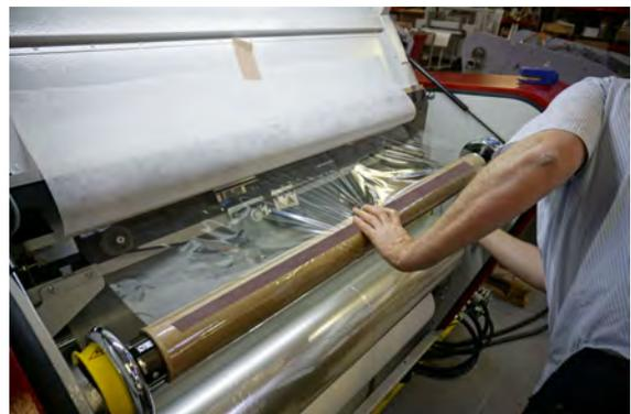
25. Loosen the nonwoven from the top cover and mount it on top of the PET on the empty waste roll.
