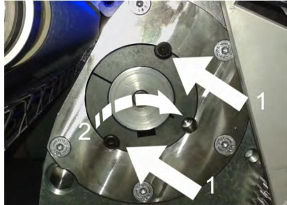
9. Remove the set screw from the taper lock.
