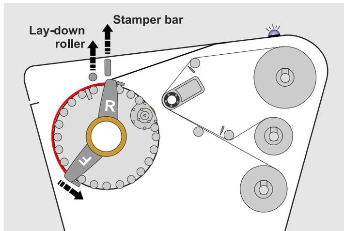
The front and rear clamp arms tension the plate ready for processing.
