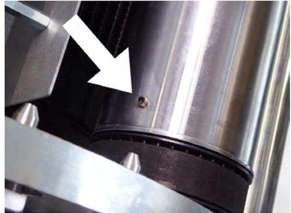
21. Mount the air hoses included with the tool kit in the two fittings in the end of the format cylinder.
