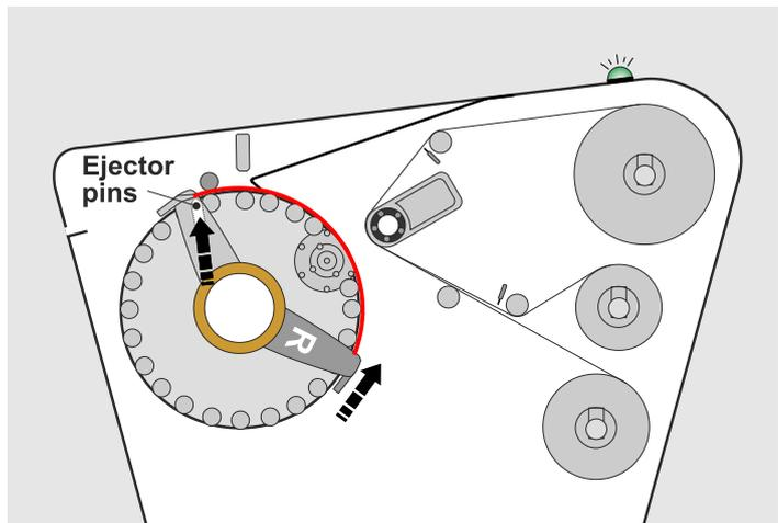
The stripping finger bar will rise to its upper position as the plate is pushed out of the processor through the exit slot.
