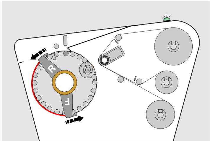
The plate rotates around the static drum for the number of revolutions defined for the selected program.
