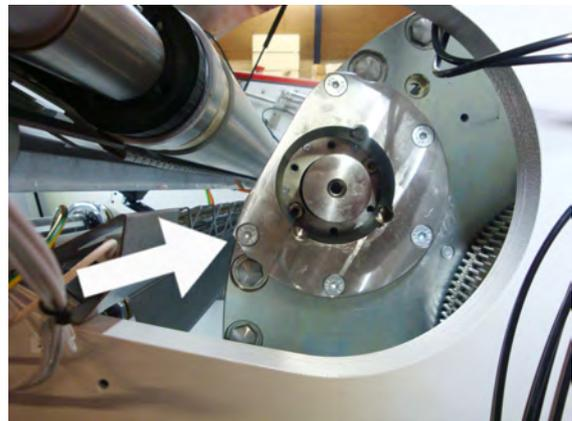
12. Remove the 4 screws from the slip fit adapter's fixation ring.
