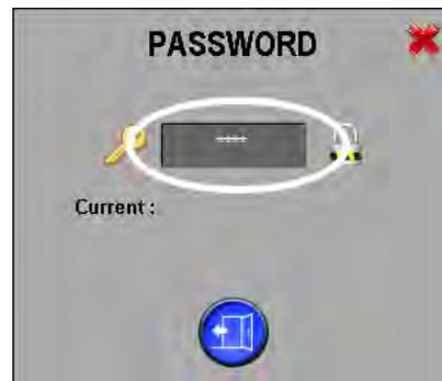
21. Touch the password input area; a numeric keypad will be displayed. Input “0” (zero). Select the “Enter” button. This will exit the “Trained Operator” level.
