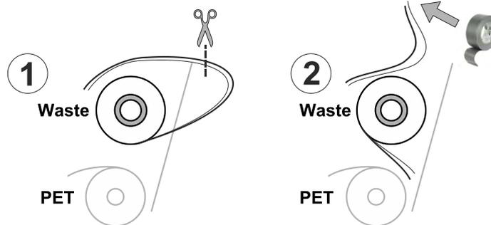
5. Fasten the cut ends of nonwoven and PET to the top cover. Each layer separately: nonwoven first and PET on top of the nonwoven.
