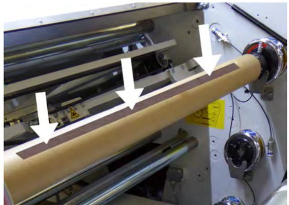
18. Loosen the PET from the top cover and mount it to the empty roll.
