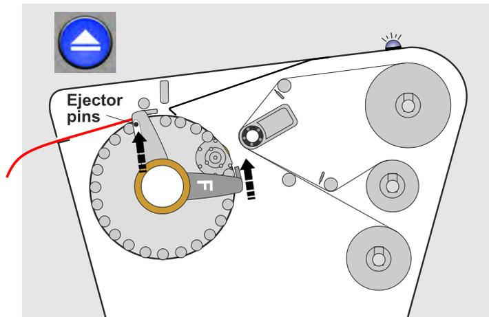
The plate will now be completely released from the clamp bar and can be removed from the exit slot.
