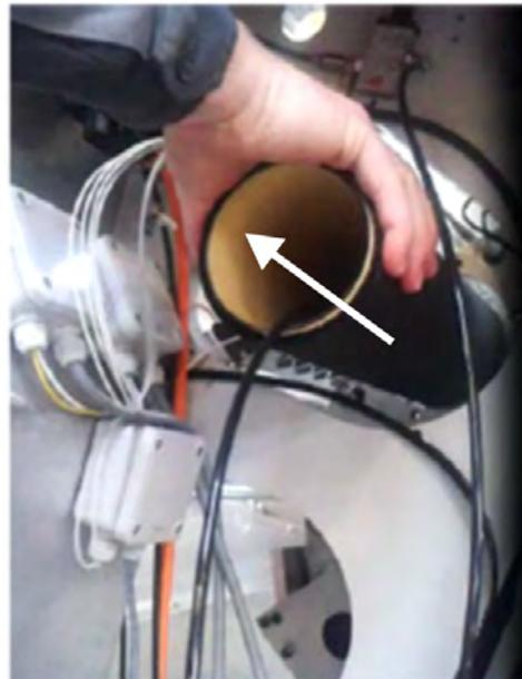
19. Turn the air pressure off and disconnect the air hose assembly.
