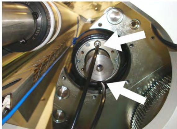
14. Locate the air switch placed on the side frame above the format cylinder.
