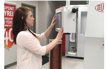
Jill Shemwell (technician, Impact Innovations) inputting the processing parameters in the Cyrel® FAST ITR processor.
