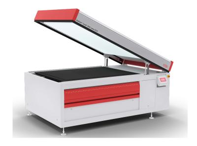
Each fluorescent tube is constantly monitored by a light guide, giving the operator a visual on/off indication. There are three-time counters imbedded in the touch screen control panel to keep track of the number of hours the UV-A and UV-C tubes have been in operation.
