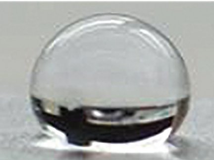
SOLDERGUARD™ 100 Treatment Before Heat Treatment
