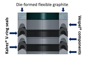
DuPont™ KVSP™ kits also can include an additional flexible graphite ring for API 607 fire safe performance.
