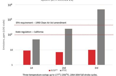
Test repeated three times according to EPA Method 21. The DuPont™ KVSP™ system maintains excellent sealing performance throughout all three thermal cycles, while PTFE valve packing tends to undergo creep at operating pressure and temperature resulting in increased fugitive emissions. The final measurement reading was around 5,000 ppm, more than 20 times higher than the EPA's 500 ppm regulation for compliance with the Clean Air Act
