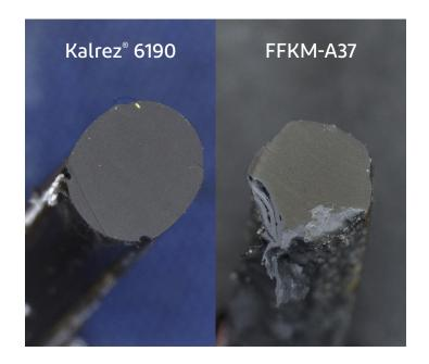
Samples of Kalrez® 6190 (at 6 months) and FFKM A37 (at 4 months). FFKM A37 experienced major degradation and leakage at the 4-month mark. Since specified, Kalrez® 6190 has been consistently reaching or exceeding 12 months seal life.
