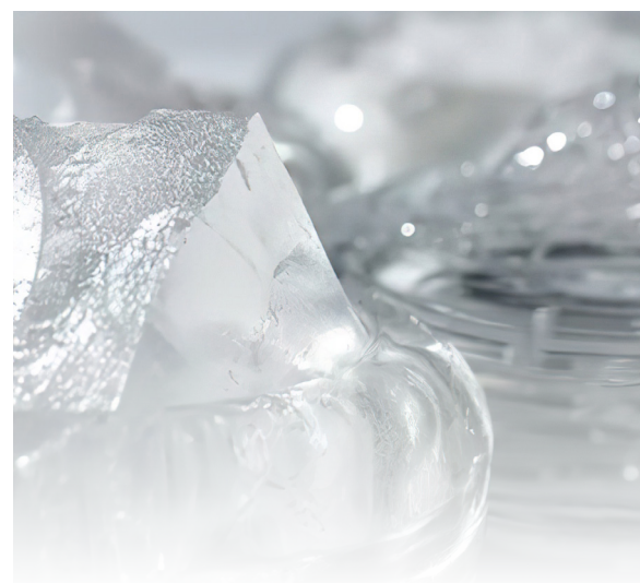
Elastomeric network swollen with carrier fluid.
