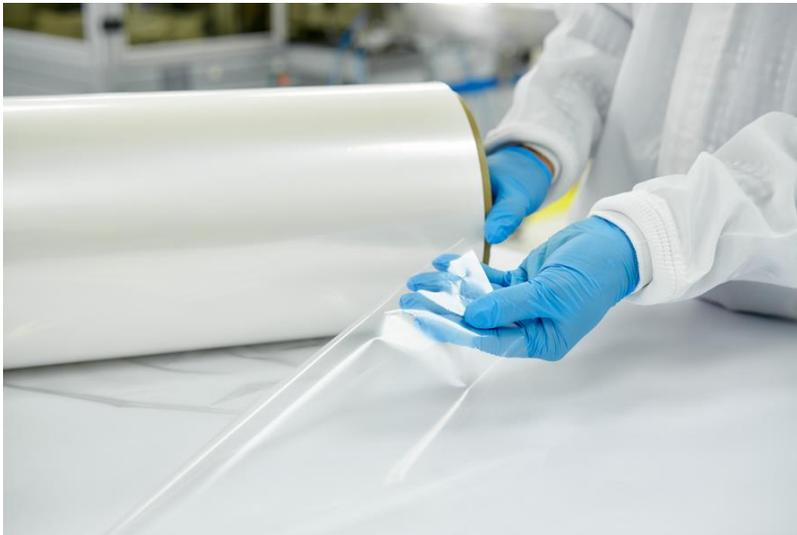
DuPont's Tedlar® film has many applications in solar panels and aerospace, but it's finding new uses as a durable, cleanable interior finish. **Courtesy DuPont**
