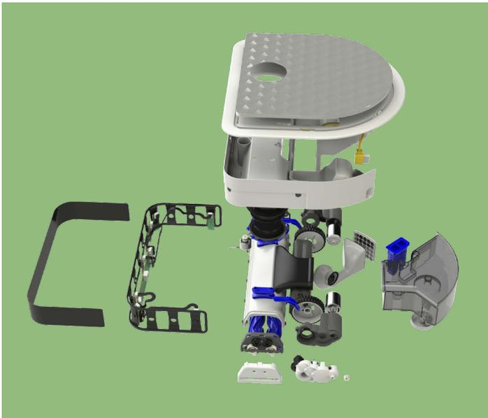
In addition to LIDAR covers and gears, DuPont materials help robot vacuum manufacturers optimize many components. This includes seals and gaskets, cleaning filaments, rollers, dampeners, motors, and connectors.
