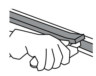
**Prepare the vehicle aperture.** If the residual PUR bead is sound and stuck firmly, trim it back to a height of 1-2 mm to provide a clean, level and secure surface for rebonding. Take care not to damage paint. Clean the aperture with BETACLEAN™ 3300 and wipe off with lint-free towel.
