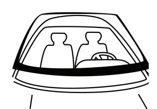
Dry fit the glass after safe removal of existing glass. Make sure the new unit fits properly and is free from defects.
