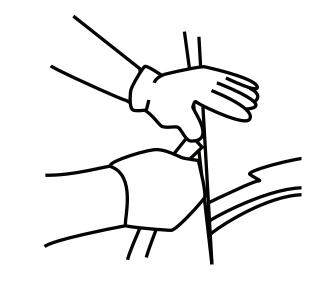
Remove all mouldings, rearview mirrors, trims and wipers, and disconnect all electrical devices and cowlings that could be impacted by cut out and installation. Open vehicle side windows and cover adjacent external and internal surfaces.
