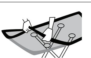
If necessary, fix continuous trim around the glass prior to installation. Be careful not to damage or contaminate the primer film.
