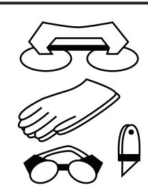
**Required materials:** Cutting-out equipment, trimming knife, glass suction, lint-free cleaning towel, primer applicators and adhesive dispenser. Ensure all products are within shelf life or open-time limitations. When opening new primer, note the date of opening on the bottle. Once open, primer is good for 7 days. Check the ARGIC code to ensure the glass specification is correct.
