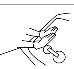
Compress the glass to the correct height within the aperture.
