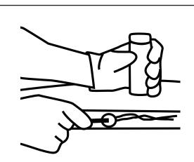
Apply BETAPRIME™ 5504G No-Shake primer to bare metal. Follow package directions and apply using wire applicator. Apply two coats of primer to build up protection. Allow a minimum of two (2) minutes for the primer to dry.
