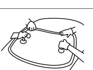
Affix the glass to the body immediately after extrusion and tooling. Take care to position the glass with minimal alignment.
