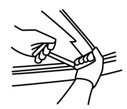
**Cut through the existing glass bond line** using your preferred method, taking care not to damage the vehicle or any electrical systems or cables.
