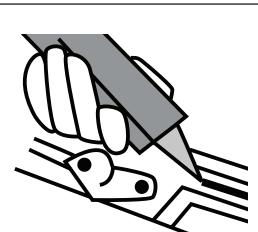
Using an 18v dispenser, apply BETASEAL™ 1585 adhesive at the bottom of the aperture or glass, using a pre-cut triangular nozzle, ensuring the new adhesive is applied over the old remaining bead where applicable. Hold the dispenser at a near-90° angle to ensure a high triangular bead. A single-only joint is preferred. Overlap the joint and
