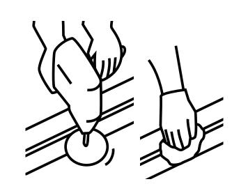
**Check for corrosion.** If necessary, grind/abrade any corrosion in and around the bond line area down to bare metal, clean with BETACLEAN™ 3300 and wipe off with lint-free towel. For larger damaged area, repair at a body shop may be required.
