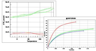
**Material card** models the influence of temperature and fiber orientation on properties
