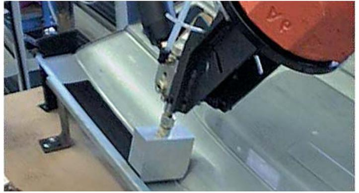
BETAMATE™ structural adhesives can be applied robotically in bead, swirl or jet spray using standard industrial equipment. The adhesives also can be applied manually from dispensing systems or cartridges.
