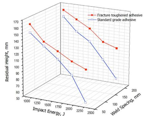
Fracture-toughened BETAMATE™ adhesives perform better than standard grades with improved stability to progressive crush and load-carrying capability.
