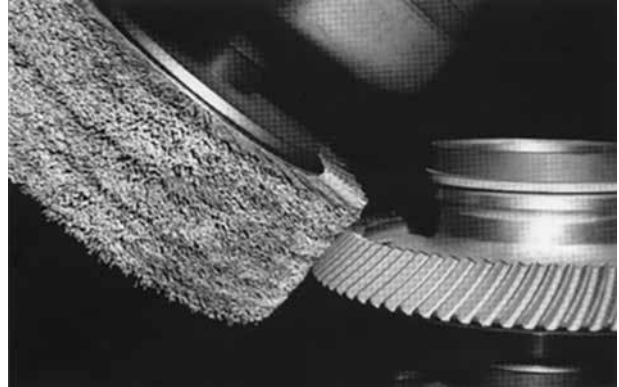
Figure 7. A Short-Trim Brush Is Used to Deburr and Finish a Gear
