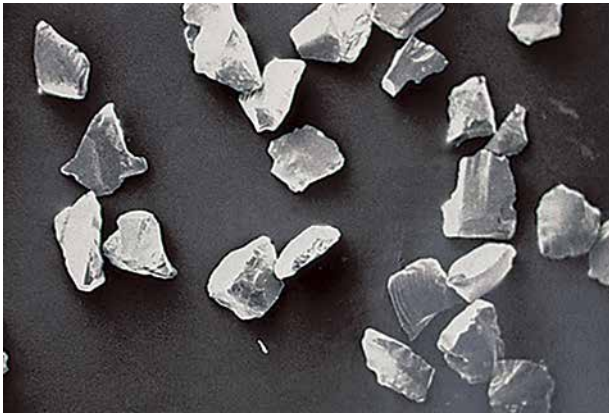
Figure 3. Magnified View of Abrasive Grit Particles
