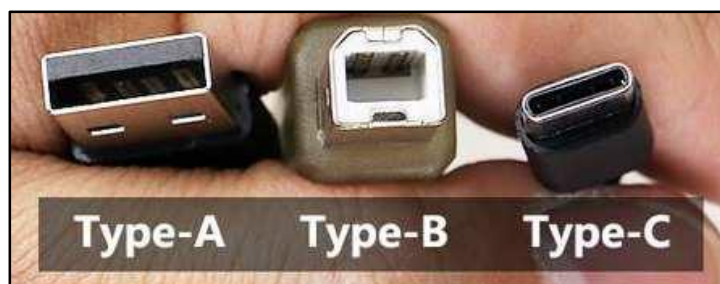
Figure 3: Evolution in miniaturization of USB connectors. Latest universal Type-C connector is encapsulated with halogen free DuPont™ Zytel® HTN polyamide, offering excellent flow rates, superior dimensional stability and low dielectric constant specifically, enabling wall thickness as little as 0.18mm.
