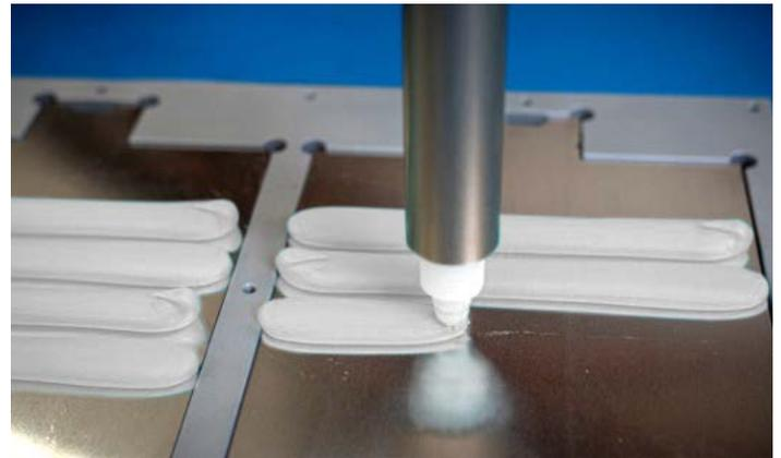
BETATECH™ thermal interface material can be hand applied or automatically dispensed for high-volume manufacturing.
