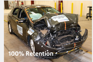
FMVSS 212 crash test of BETASEAL™ adhesive primerless-to-glass urethane adhesive after 30 minutes of cure.
