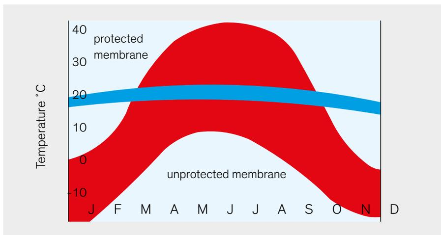
Figure 1: Temperature fluctuations in an unprotected roof covering compared with those in one protected by XENERGY™
