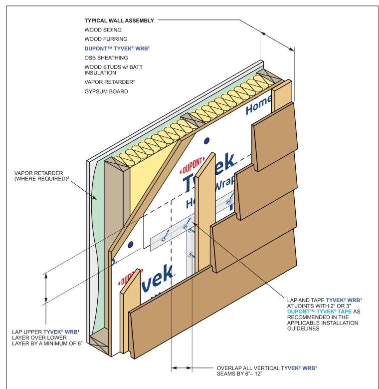
REFER TO THE FACADE CONSIDERATIONS SECTION OF THE APPLICABLE DUPONT INSTALLATION GUIDELINES TO HELP DETERMINE THE APPROPRIATE TYVEK® WRB FOR THE CLADDING TYPE.
