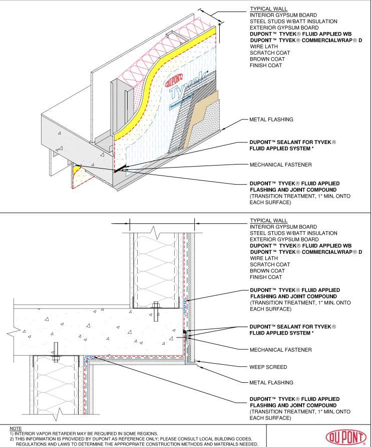
\* DUPONT™ SEALANT FOR TYVEK® FLUID APPLIED SYSTEM OR DUPONT™ TYVEK® FLUID APPLIED FLASHING AND JOINT COMPOUND MAY BE USED.
