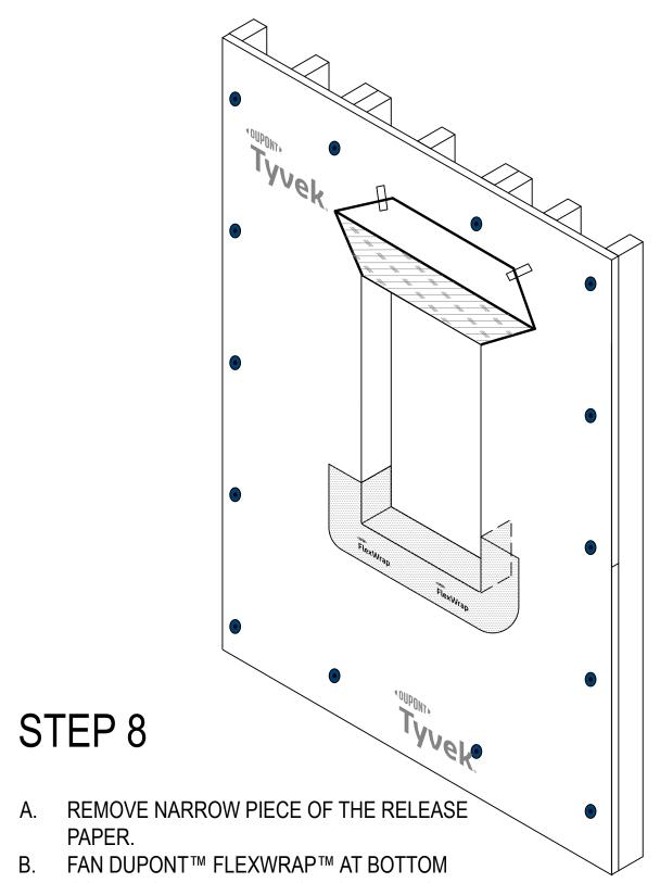
B. FAN DUPONT™ FLEXWRAP™ AT BOTTOM CORNERS AND ADHERE ONTO EXTERIOR FACE OF WALL. COVERAGE SHOULD BE 2" TO 3" INCHES ONTO THE FACE OF THE WALL
