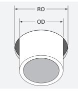
Use **FlexWrap**<sup>™</sup> **EZ** only when penetration rough opening (RO) is not more than 1/2" larger than the outside diameter/dimension (OD) of non-flanged product.
