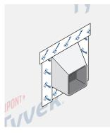
STEP 5 Seal edges of **Tyvek**<sup>®</sup> **WRB** with Tyvek<sup>®</sup> Tape.
