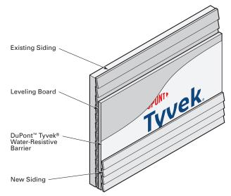
\*Use **DuPont<sup>™</sup> Self-Adhered Flashing products** with **DuPont<sup>™</sup> Adhesive/Primer** (or recommended primer) as applicable to seal the **Tyvek**<sup>®</sup> **WRB** directly to concrete, wood, or other rough surfaces. The **Tyvek**<sup>®</sup> **WRB** can also be sealed to rough surfaces
