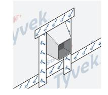
STEP 4 Seal seams using Tyvek® Tape.
