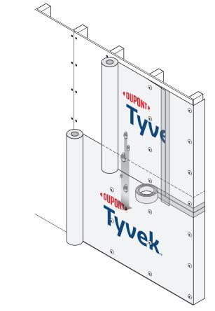
A. Lap all components from bottom of the wall to the top of the wall.
