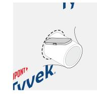
STEP 1 Install **Tyvek<sup>®</sup> WRB** over non-flanged product and cut around penetration.
