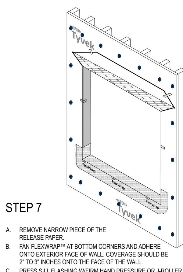
C. PRESS SILL FLASHING W/FIRM HAND PRESSURE OR J-ROLLER TO ENSURE FULL ADHESION ON ALL SURFACES.
