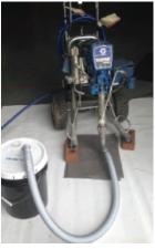
Regardless of which method is used, the delivery equipment should supply a sufficient volume of product to avoid "starving" the system and spraying should be discontinued before the level of the **DuPont™ Tyvek® Fluid Applied WB+™** runs low to avoid the introduction of air into the system. The spray equipment manufacturer can be contacted for additional information about operation guidelines and recommendations based on the material properties and constraints provided.
