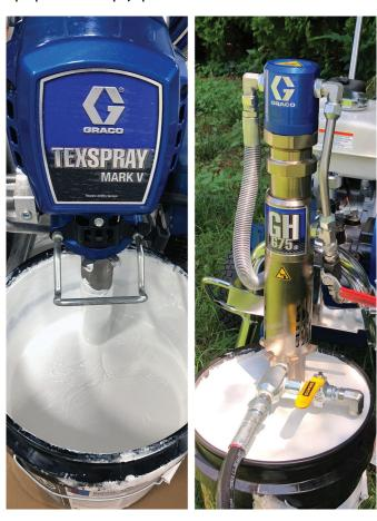
A transfer pump is another great option for delivering **Tyvek® Fluid Applied WB+™** from the 55-gallon drum to the airless sprayer. The transfer pump creates suction pressure to enable a continuous flow rate with lower pressure drops during the extraction of higher viscosity products like **Tyvek® Fluid Applied WB+™** from the 55-gallon drum to the airless sprayer.
