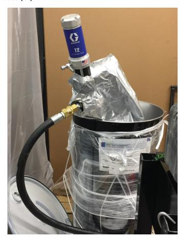
The third and final option for extracting DuPont<sup>™</sup> **Tyvek® Fluid Applied WB+™** from the 5-gallon bucket and 55-gallon drum is through a siphon.
