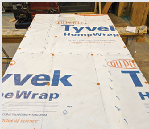
The Wall Assembly with DuPont™ Tyvek® HomeWrap® Tested per ASTM E2273 Exhibited a Drainage Efficiency of >90%.
