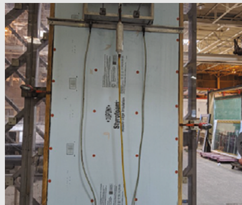
The Wall Assembly with DuPont™ Tyvek® HomeWrap® Tested per ASTM E2273 Exhibited a Drainage Efficiency of >90%.
