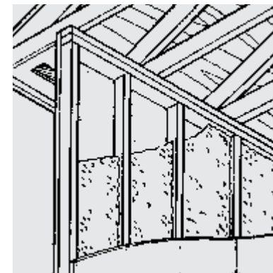
Figure 8: Insulating stud wall cavities (maximum 2" [50 mm] thickness)
