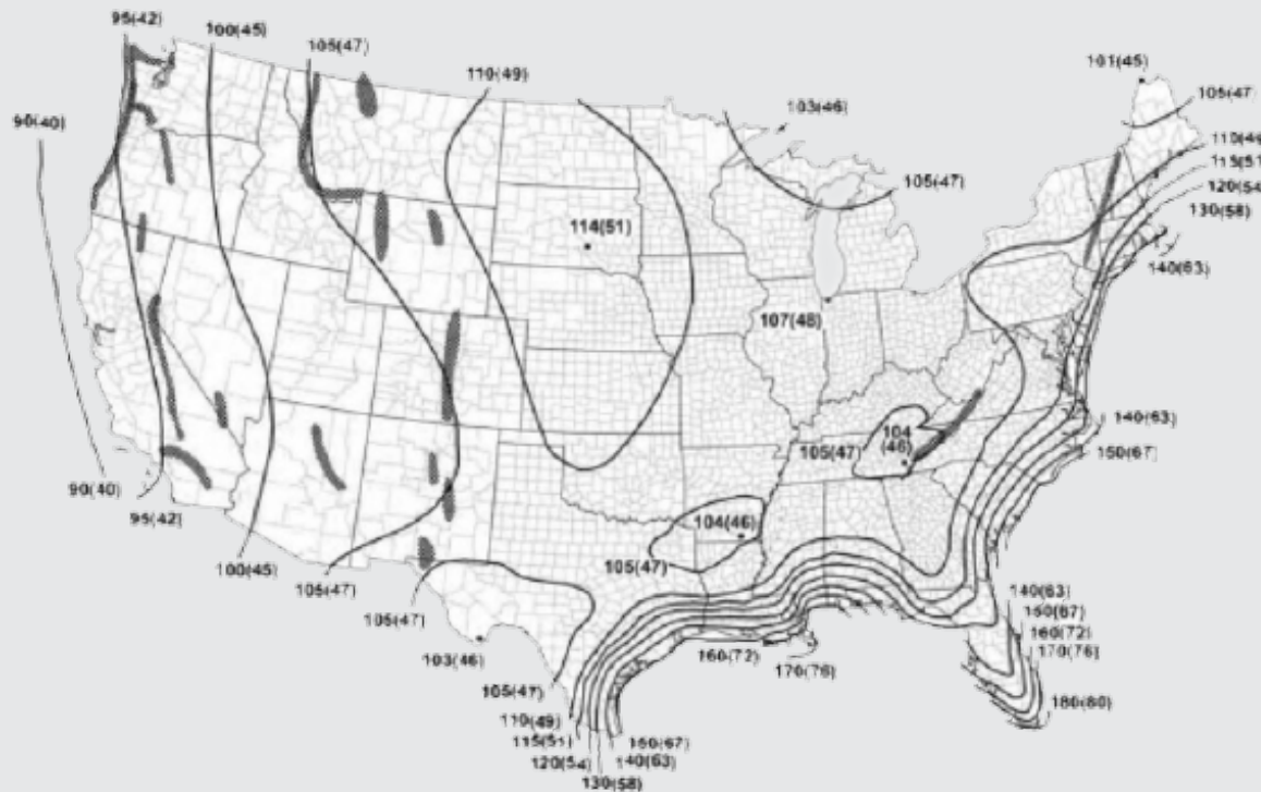
Figure 3. Basic Wind Speed – ASCE 7-16 – Exposure C - Category II
