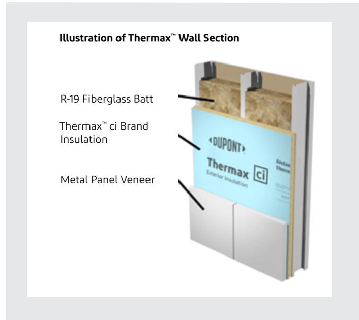
Thermax™ Insulation Wall Section – R10 CI (1.55”) + R19 Cavity
