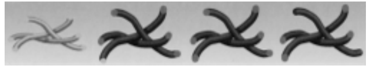
Figure 3.1 Representation of thickening of Nomex® III when exposed to heat and flame, in accordance with ISO 17492 TPP testing
