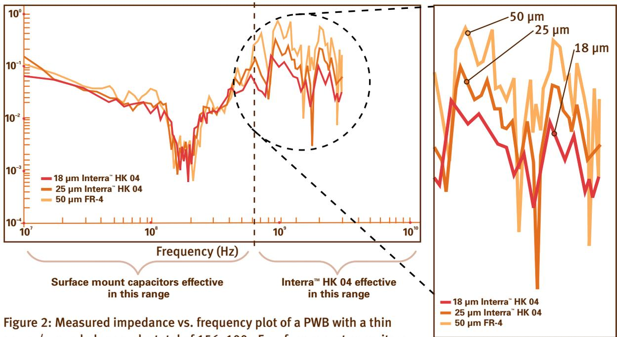
Figure 2: Measured impedance vs. frequency plot of a PWB with a thin power/ground plane and a total of 156, 100 nF surface mount capacitors.
