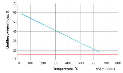
Note: LOI is the measure of a materials combustibility. 21% oxygen is the defined as the flammability threshold for ambient conditions. Graph shown for 5mil thickness.
