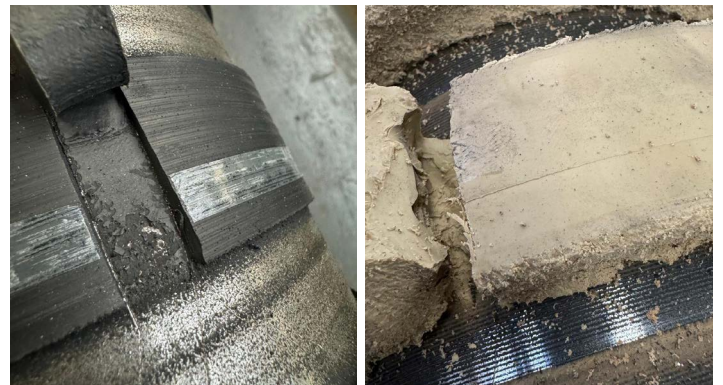
Test results show superior bonding performance of MEGUM™ W-Series specialty adhesive for both hard and soft rubber to metal and aluminum rollers.
