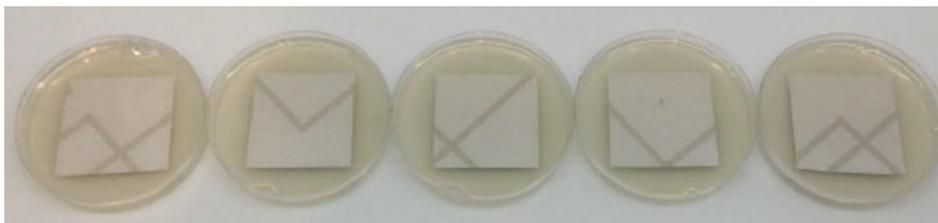
No bacterial growth in the agar or around the specimens. The specimen does not contain nutritive components.
