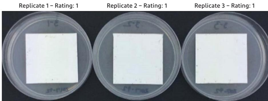
**Figure 2:** White Tedlar® PVF film (TWH15BL3) after four weeks of incubation in the ASTM G21 test. Trace growth was visible and additional growth was visible at 20X magnification.
