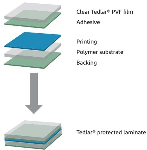
Figure 1: Picture of Tedlar® PVF film and a schematic of a laminated structure including Tedlar® as a protective surface glazing
