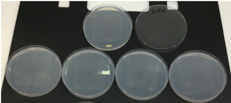
No bacterial growth in the agar or around the specimens. The specimen does not contain nutritive components.
