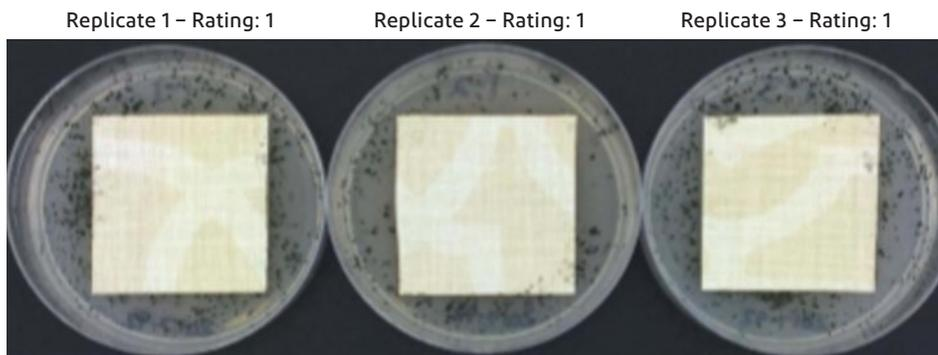
**Figure 3:** DuPont™ Tedlar™ Wallcovering after four weeks of incubation in the ASTM G21 test. Trace growth was visible and additional growth was visible at 20X magnification.
