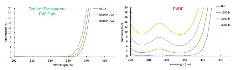
UVA Test: UVA-340 fluorescent bulb, 1.2 W/m²-nm @ 340 nm, 70 °C black panel temperature. Each 1000 hrs provides 65 kWh/m² of UV light from 290 to 400 nm.
