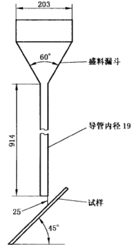
**Falling sand abrasion resistant Test**
