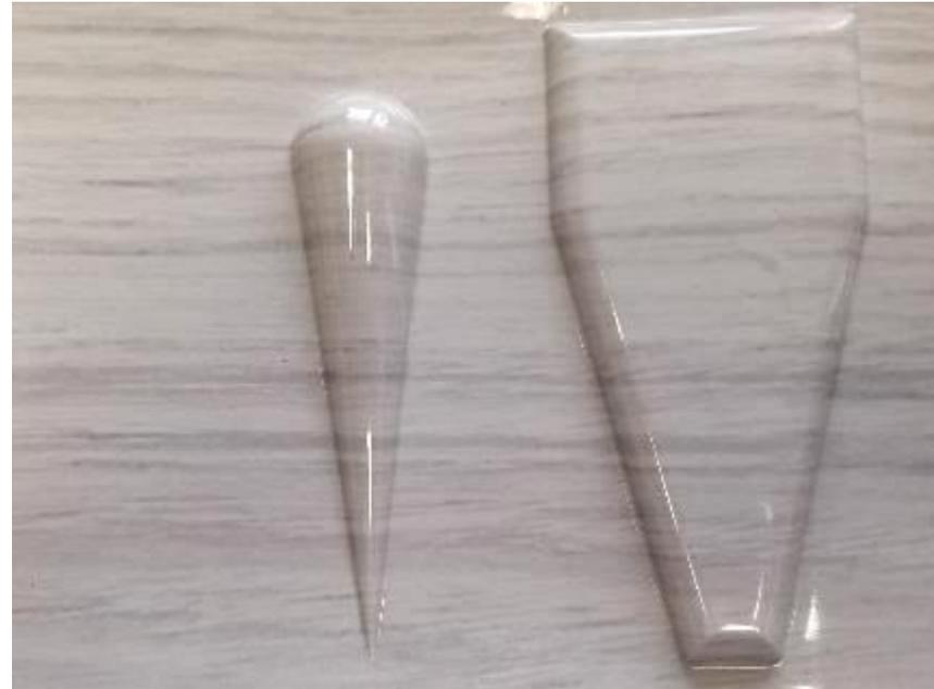
**Tedlar® film is thermoformable, expanding the use of the material beyond flat surfaces.**
