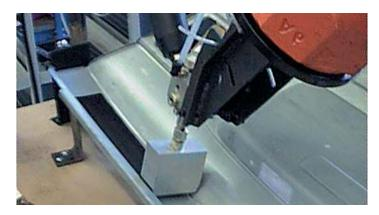
BETAMATE™ structural adhesives can be applied robotically in bead, swirl or jet spray using standard industrial equipment. The adhesives also can be applied manually from dispensing systems or cartridges.
