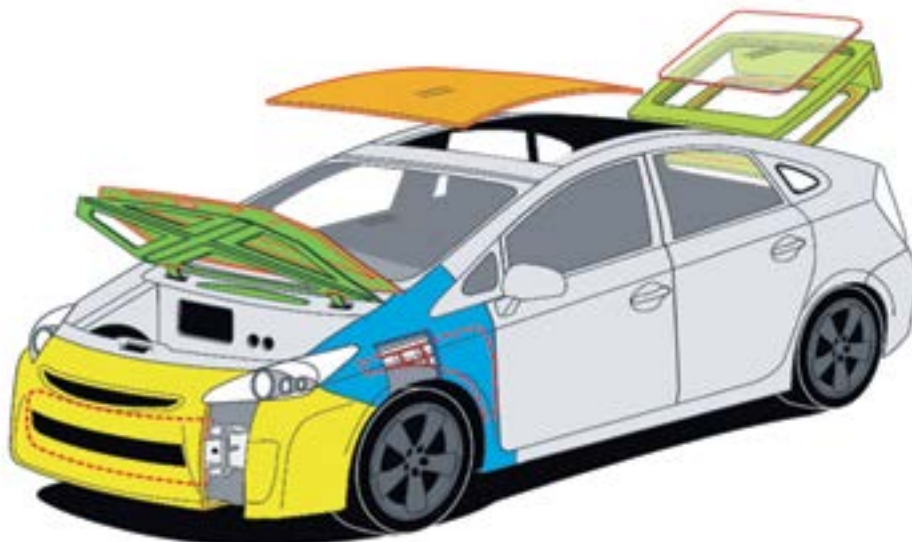
Figure 2 - Potential application areas of bonded hybrid composites.
