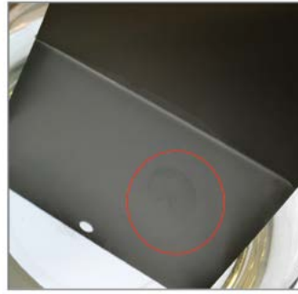
Picture 5c: immersed metal plate with finger print contamination
