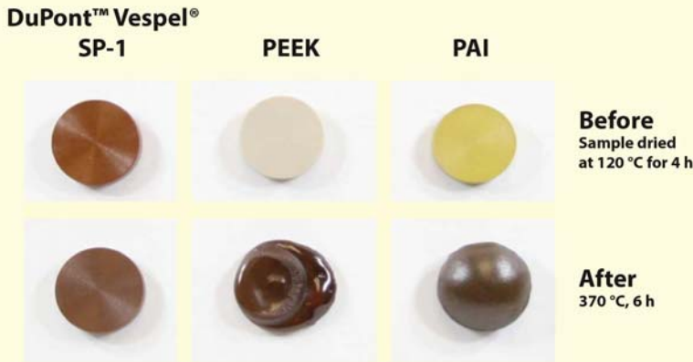
Fig. 5. The illustration demonstrates the deformation of pure unfilled PEEK and PAI resins after exposure to 370°C for 6 hours, while pure unfilled Vespel® SP-1 remained unchanged. PEEK will soften at 140°C while Vespel® remains essentially unchanged at 350°C+. In addition, Vespel® parts continue to support high loads at this temperature, unlike PEEK.
