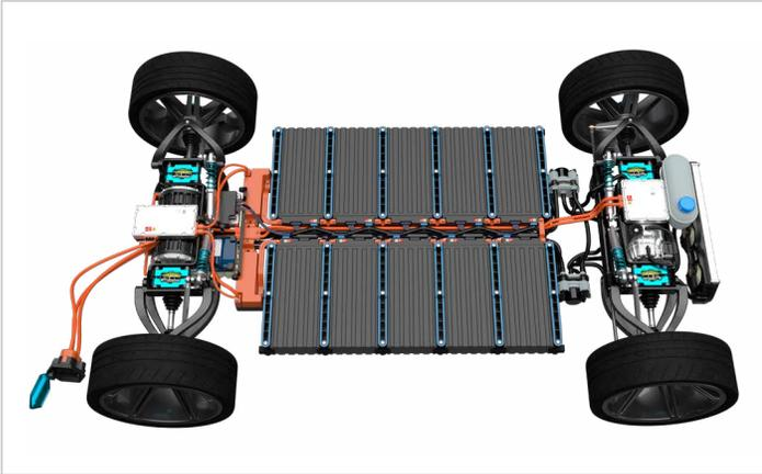
Automotive cooling lines (also known as pipes, tubes, or hoses - often combined with connectors) are a well-known application for thermoplastics and elastomers. These systems are found in all types of vehicles regardless of the type of propulsion. But in EVs, cooling requirements are elevated.\* As a result, the cooling lines themselves can be up to three times the length of those needed for ICE vehicles.
